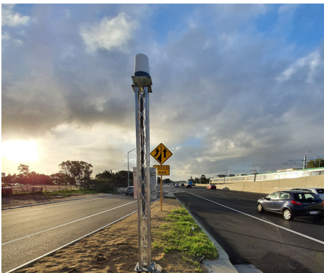
Kwinana Freeway, Australia 13 radar installed Across 13km freeway
